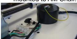
2) Plug the Molex Connectors from the Transformer and the Dental Light (coming from bottom of light post).
