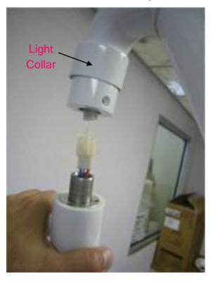
7) Slide the connectors into the Light Arm and Light Head.
